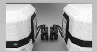
Two or more vehicles would automatically line up together using position sensors.
