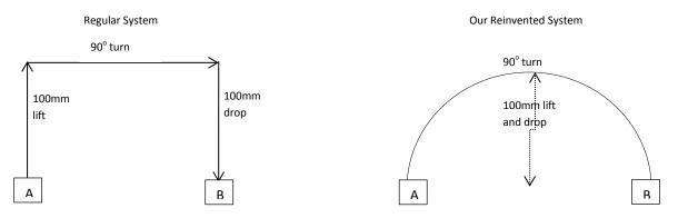
Using the new system would shorten the time of lifting and dropping by completing the task in the centre of the  $90^{\circ}$  turn. The brief would be satisfied, but performing it in one smooth action in comparison to three, cutting the transaction time too for each action.
