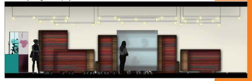
In the main gallery, there needed to be a way to display paintings on the curved unit. This was solved by adding a track to the top, so that paintings could hang on the units without damaging the display itself.
