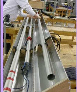
The larger part of the mast went in the top section by itself, a bar comes across to make sure it doesnt fall out when the tube is closed.
