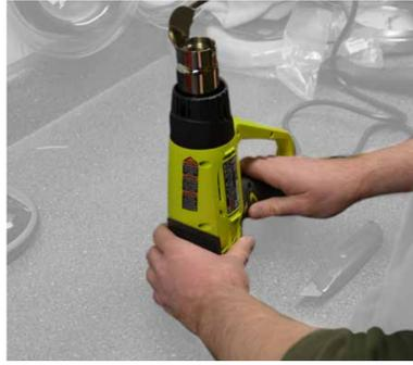
The Ryobi heat gun was not very stable when it was sitting on its end, this was extremely onconvenient for bending pipes.
