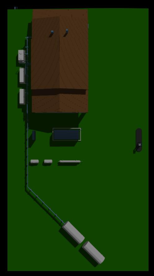
The FirmGreen Columbus, Ohio Site was laser scanned and modeled in 3D utilizing the latest technology available. 20 Individual 360 x 310 degree laser scans were captured at an accuracy level of 5mm across a span of 50m. The laser Scanner generated 500,000 vector points of true x,y,z coordinates applied per second of operation. This vast amount of 3D points is what the industry labels 3D Laser Point Clouds or Scan Worlds.
