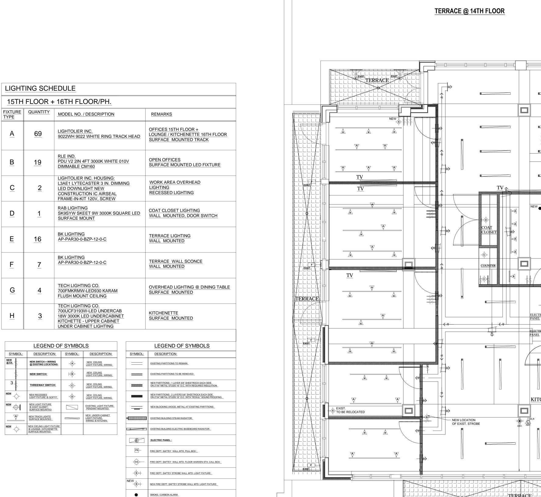
LIGHTING, SWITCHING, WIRING - CONSTRUCTION -15TH FLOOR PLAN
