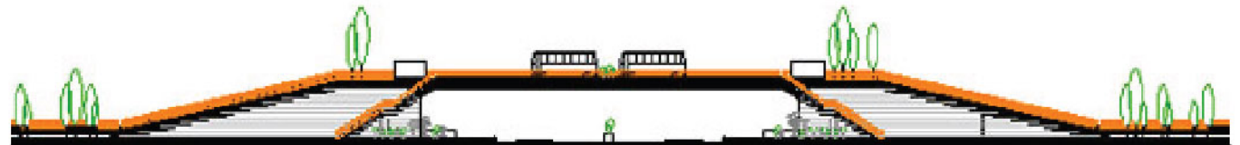
Schematic Section: Segregation of Highway road and Local road. Also linking the local roads on opposite sides of an highway
