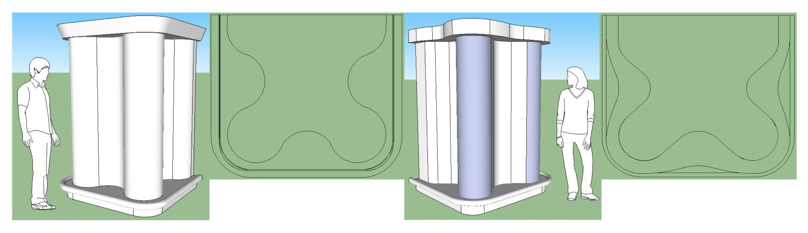
Two versions of an end cap made in Sketch Up. In order to increase product space using the same footprint the 3 walls were pushed inward. It would be useful for small hanging blister packs or it could be configured for sunglasses.
