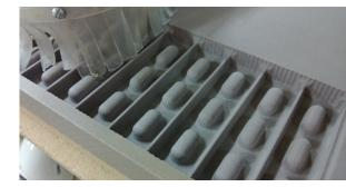
Machining the "Buck" that would be formed over.
