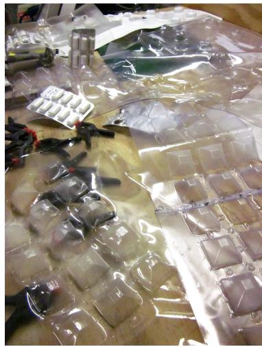
Dozens of mock ups were made in order to test the structure and usability of different shapes and materials. This was one of the most critical phases of the project because it dictated the final shape of the product as well as what material should be used and in what thickness.
