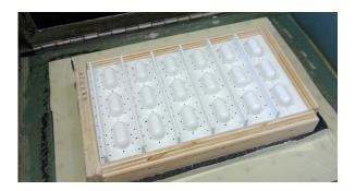
Hundreds of small holes were drilled into key areas of the "Buck" to insure that the material formed correctly around each detail.
