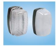
The lantern is a Coughtrie BD model, sat loose on top of the base. It is made from die cast aluminium and features a matt black textured case. There are a range of power options, from 9W to 2x13W, and the lantern is IP65 resistant, which means it is completely sealed from dust, and sealed from low pressure water jets. It uses a florescent low-energy light source
