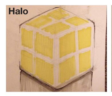
Top is replaceable, wipe clean surface Plastic will be susceptible to denting and puncture Retains square lighting, with modernist touch. Can retail original frame, rotational moulding is not the best for very small scale production.
