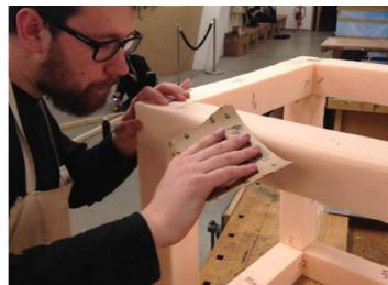
The frame was supplimented by glued wooden 'window frames' which would hold on the sheets of plastic. I taped cardboard crosses to simulate the boxes. All of the geometry checks our, the cardboard crosses are a 45 cm square, which is equivalent to the inside faces of the steel box. the edges of the model are 60 cm out, which corresponds to the 598mm wide CAD model.
