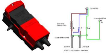
The light is wired in to the three common power wires - earth, live and neutral. The red device is a TOFCO F114 Fuse unit, which puts the electricity supply through a fuse and connects it to a lantern. These are ubiquitous devices which can be easily re-sourced in necessary.
