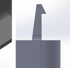
I have kept the wall thickness at around 2mm throughout the both parts, and attempted smooth transitions.
