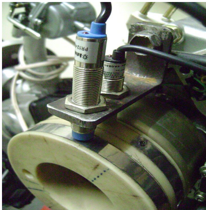
Figure 3.5 Installation of Sensors
