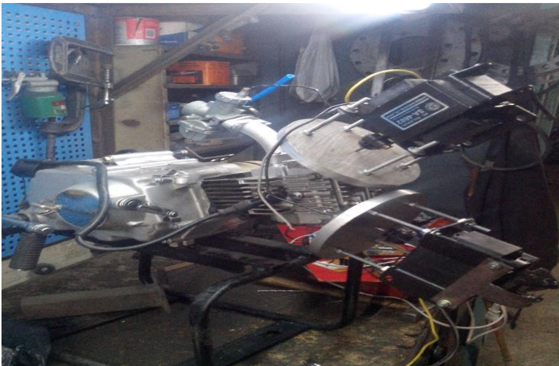
Figure 3.4 Installation of Solenoids
