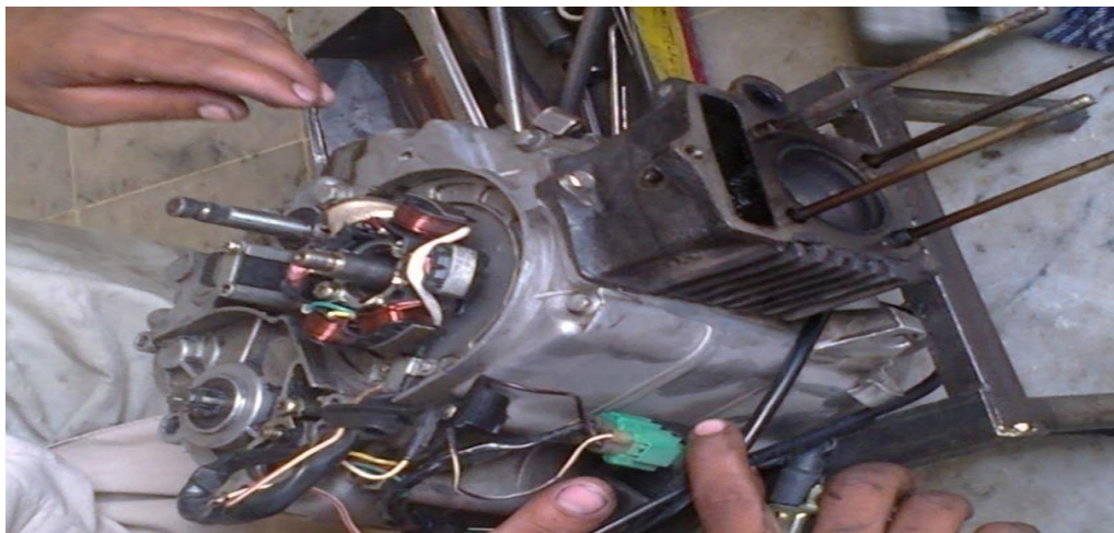
Figure. 3.1: Removal of Head Engine
