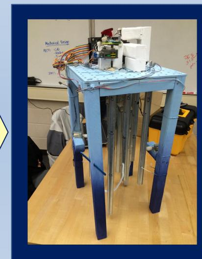
Going off of our previous CAD we decided to rearrange our chimes and incorporate stationary solenoids to help with timing of the song and we also decided to save material by only leaving enough wood material to hold the solenoids on the side.
