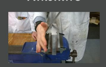
Lastly the mould block and inserts had to be finished using a file and wet and dry paper to ensure no bumps or marks will show up on the injection moulded product. This included any imperfections. We also used air blaster to prevent dirt from being mixed with the polymer.
