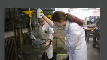
We used the drilling machine on the two mould blocks to ensure the alignment pins fitted securely in place. This included drilling the hole and reaming it to M6. We also drilled a hole beneath the main round insert to make the removal of the insert easier.
