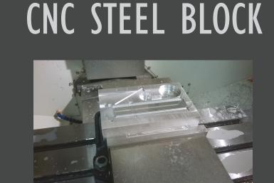
Once the blocks of steel were carefully aligned in the CNC machine the mould could then be machined. From this the internal tolerances could be checked to ensure the inserts will fit accurately into the cavities.
