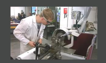
In order to produce the two round inserts and the two main alignment pins we had to use a centre lathe. For the inserts we turned and faced off the aluminium down to size in order to fit the correct tolerance in the mould. The pins were turned to create a chamfer on the end, this is to make inserting the pins easier and for de-burring.
