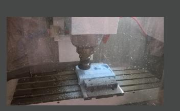
Before the steel blocks can be cut on the CNC machine the coding and CAD model firstly has to be tested using blue foam. This will highlight any issues or problems that need to be changed with the programming such as feed rate, sequence and the timing.
