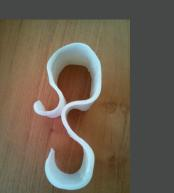
Models were produced to gain further understanding of the product, size, proportion and the feel of the product which can then be assessed for further development. Both models are important to the design process: the clay model for initial changes and the 3D printed model for an accurate representation of the final
