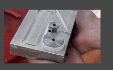
Once the inserts and mould were accurately completed the product could then be injection moulded out of the two halves using LDPE plastic. Firstly with white as this has the lightest pigment and then all the way through to black.
