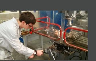
The milling machine was used to cut the middle insert to size and face off the mould blocks so that they are square and sit flush in the injection moulding machine.
