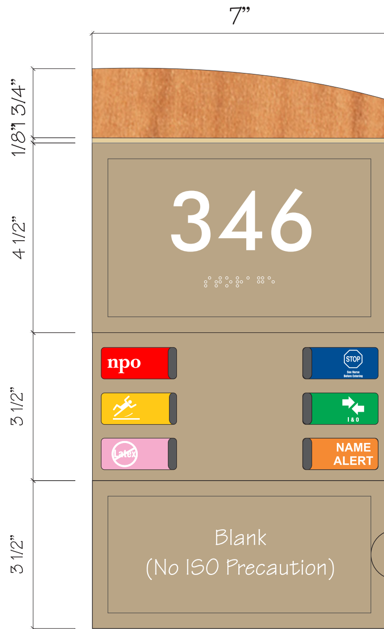
Module 3.7-ID 6-Slot Patient Precaution Slider w/Isolation Precaution Frame
