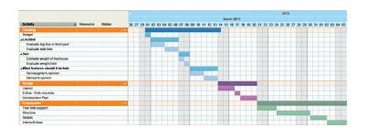
(WBS); a method of organizing tasks into a manageable schedule. The WBS combines several parts which creates a time-line that describes how to move through your project. The example
