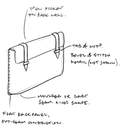
TAS SHAPE PRINOUNC 6D OUT-SCAMSTITCH A GTAIL WITH FLAT BASE TAB & LOOP WITH BEVER DETAIL (NOT SHOWN).
