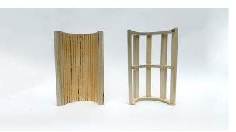
While kerfing was successful for some pieces, we found that it failed for others. the vertical step support needed to be redone in order to become lighter and more precise. We created a ribbed wooden frame the second time around.
