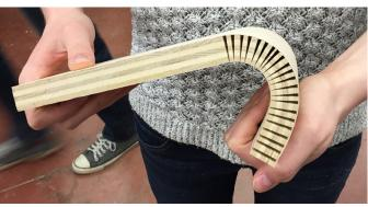
In order to achieve the curved wood surface, we decided to use a cutting method called kerfing. This process cuts away most of the wood, allowing the top veneer surface to become highly flexible.
