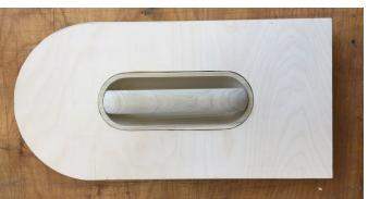
The handle was cut by a CNC mill so that pure angles and curves could be achieved. The holder that the handle fits into was also milled. We cut the corresponding shape into the lid by hand so that the pieces could be fit together.
