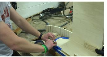
The cut pieces were then clamped around rounded templates to create the appropriate size curves. After clamping the pieces, we poured glue inside of the cuts until they filled and dried in place.
