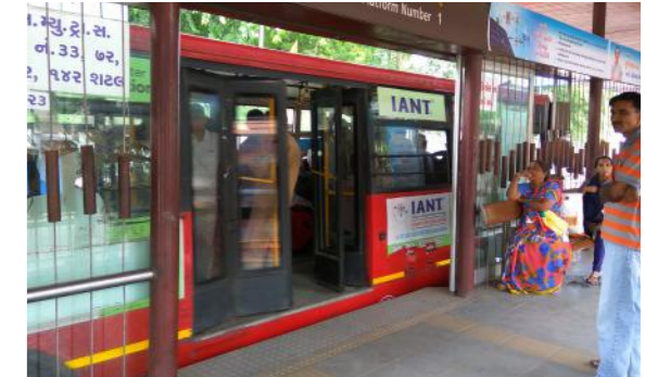
Automatic doors in AMTS feeder buses
