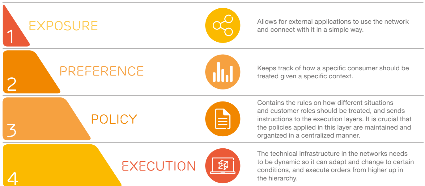
Figure 4: Programmable networks: a tiered architecture
