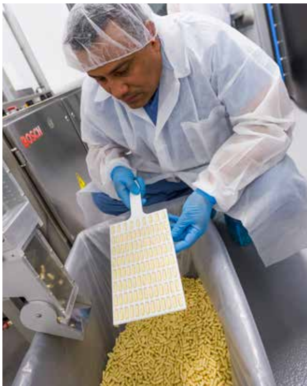
Encapsulation machines produce between 50,000 and 100,000 capsules per hour. That's up to 50 million capsules each month!
