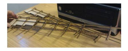
We chose the GOE 239 profile for its high lift to low speed ratio. The design accomplished 4.3 amps and managed to light 2 light bulbs whilst still rotating. Our calculations showed that it would be effective in reaching our goal of little drag, high lift and powerful torque.
