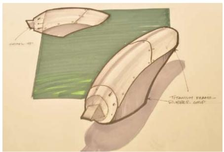
The proposed materials that I mentioned in the Rapid Visualization phase was a titanium frame shell, a rubber grip, and a chisel tip.
