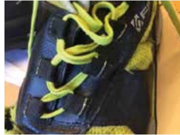
LACING SYSTEM WAS NOT ERGONOMIC WEBBINGS BREAK, EYESTAY WAS NOT FUNCTIONAL
