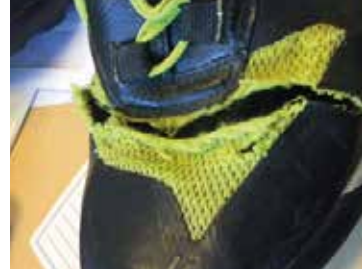
NEW MESH MUST BE DURABLE AND TIGHT-WOVEN ENOUGH TO KEEP FINE SAND OUT
