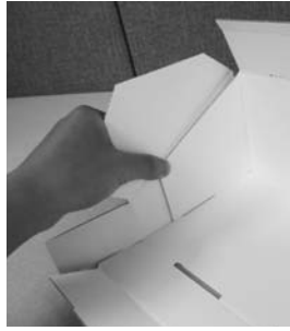
Step 2 Fold the back up and the tab inward. Fold the side up and bend over the tab, locking the side into the bottom cutout. Repeat on the other side.
