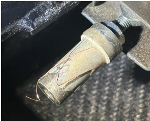
Rear Toe-Link Bond failure on CF-Resin interface during on-track testing. (Sudden rupture during forward accel)
