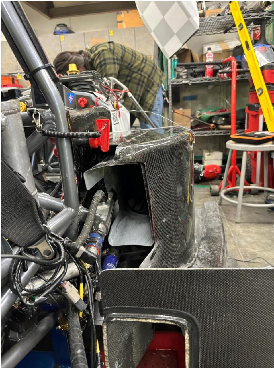
Outlet Duct with cutouts to allow for Oil Cooler fitment and flush sidepod mounting
