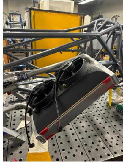
Verifying Radiator Angle
