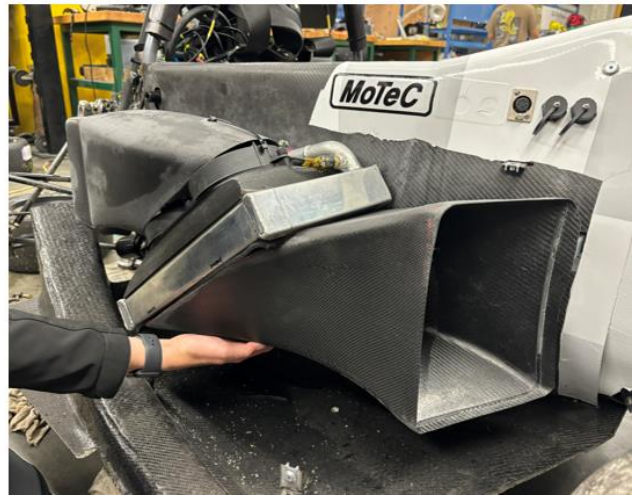
Final Ducting Mock-up
