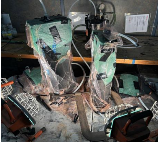
CF ducting via Resin Infusion
