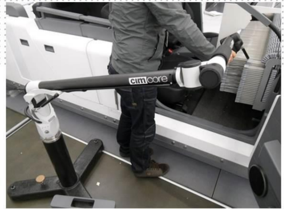
3D measure to check changes
