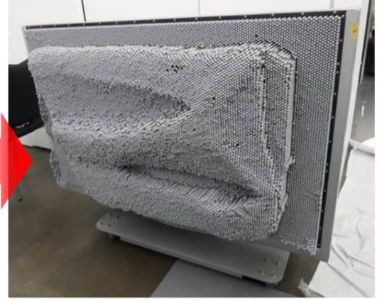
Construct a pin module molding using the vehicle exterior gauge when considering the door review
