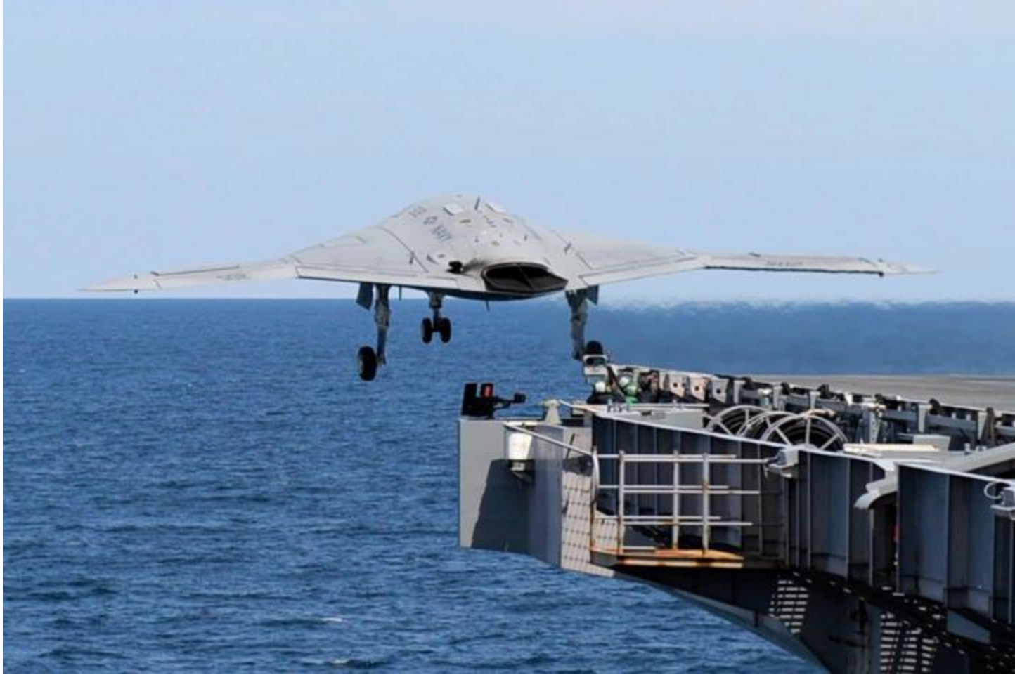
An X-47B demonstrator launches from a catapult aboard the aircraft carrier USS George HW Bush in 2013. The X-47B project proved that unmanned aircraft with fully stealthy shapes could operate from US carriers - Alan Radecki/US Navy/Northrop Grumman
