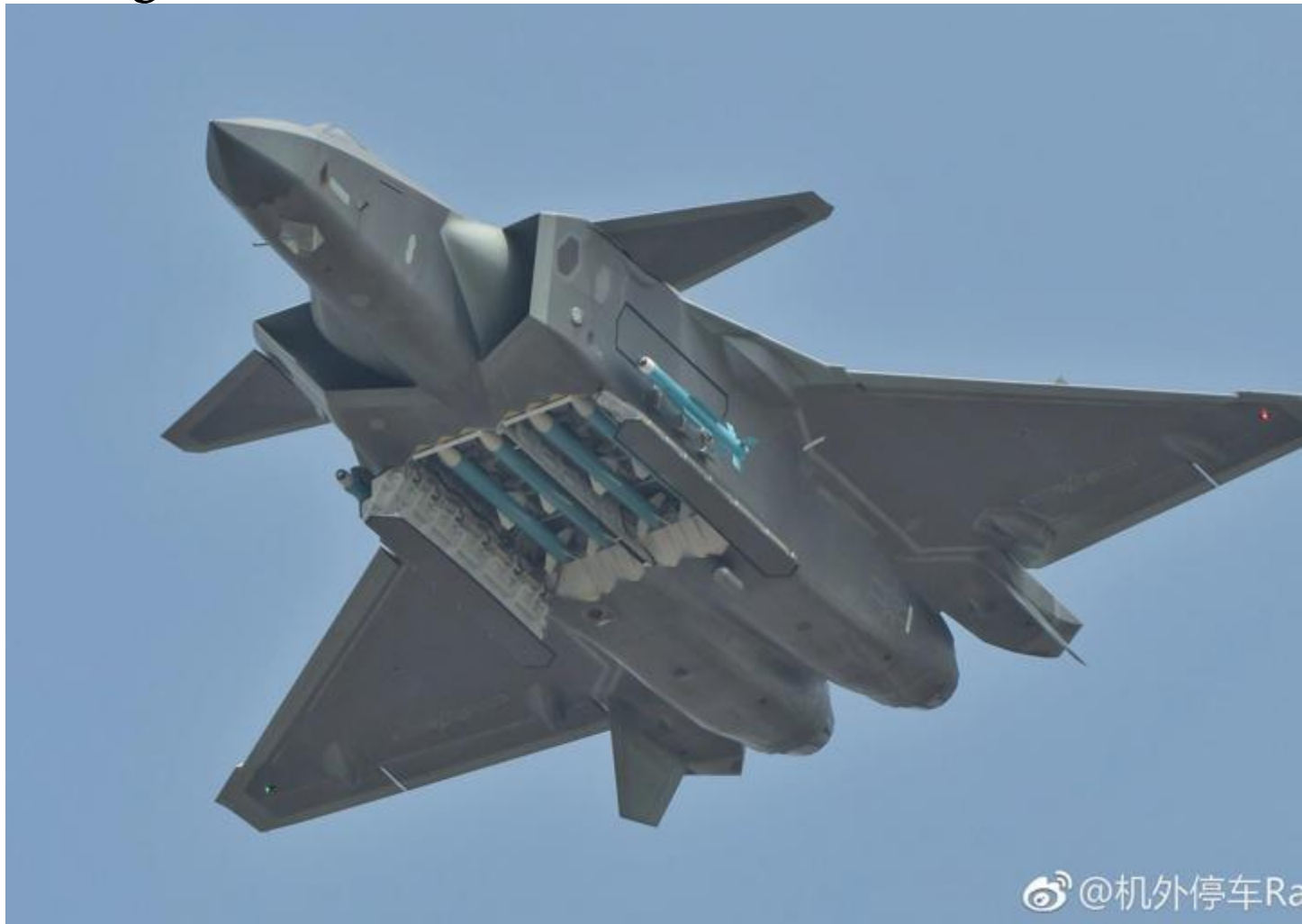
A J-20 flying overhead during the 2018 iteration of the Zhuhai Air Show, displaying its internal weapons bays with a full load. (Image credit: Telegram/Sina Weibo)
