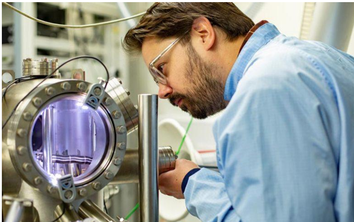
Dr. Taylor Stock loading a sample into the scanning tunneling microscope (STM), used to perform atomic scale fabrication. Credit: Agnese Abrusci/UCL.
