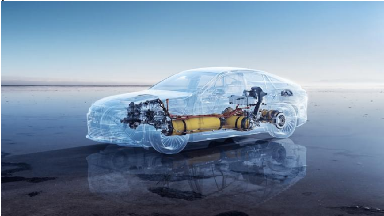
graphic depicting the inner workings of a 2024 Toyota Mirai, showing the vehicle's hydrogen storage system, fuel cell, and electric motor.© Credit: Toyota
