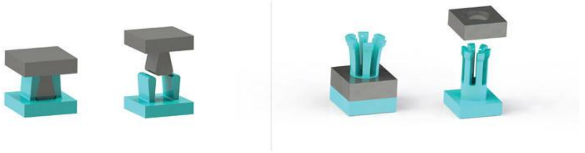
An individual cell of the two proposed versions of ILMs in their different engagement states. Credit: Dr. Ibrahim Karaman
