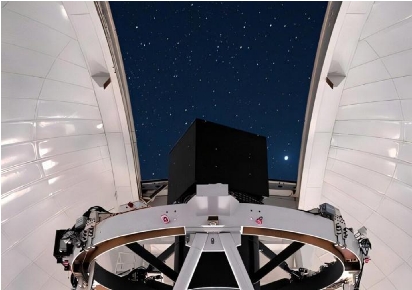
The WEAVE prime-focus corrector and positioner at the William Herschel telescope in La Palma, Spain. Credit: ING
