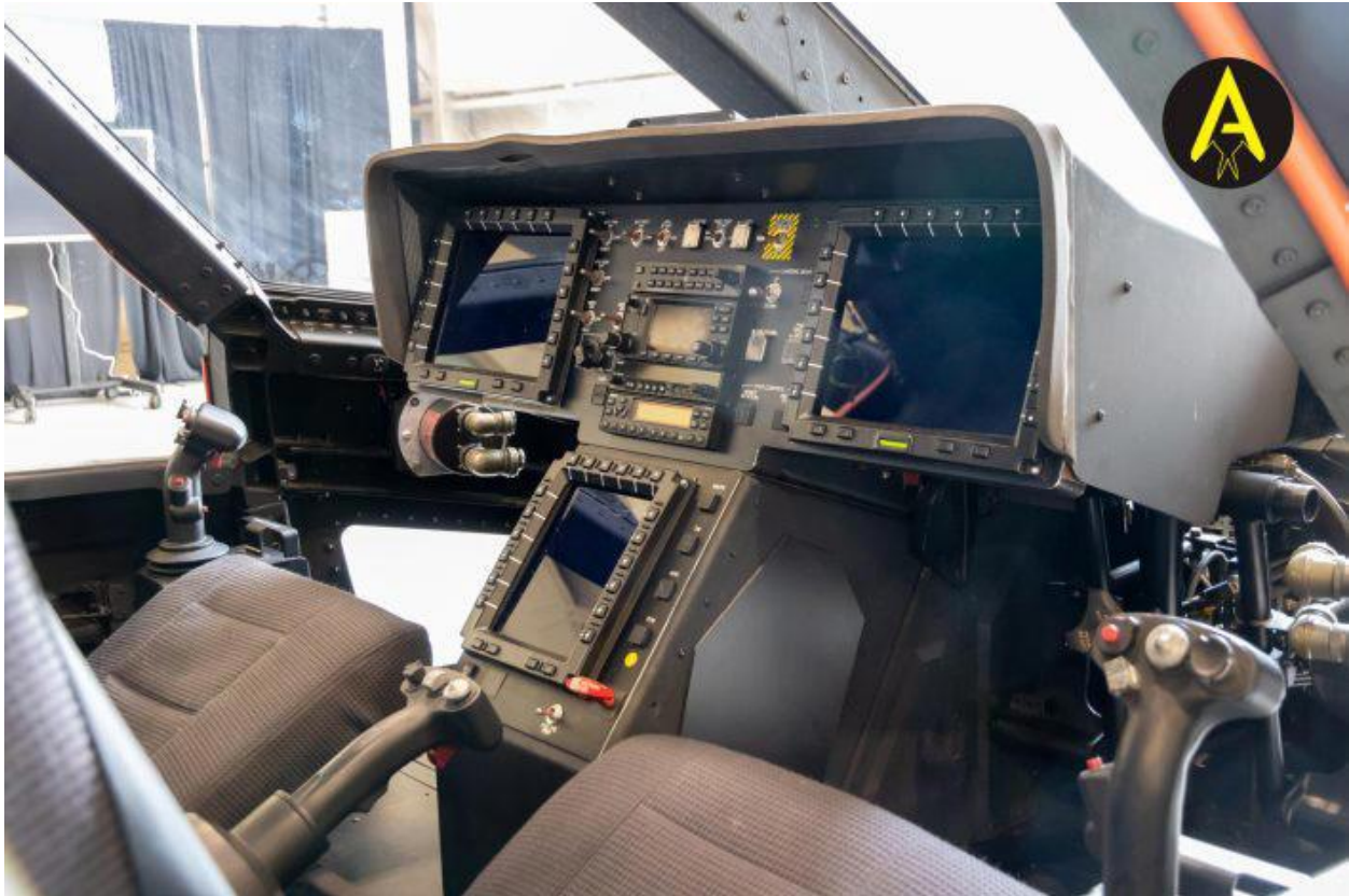
The cockpit of the S-97 Raider, with the two sidearm controllers and the single collective visible.
