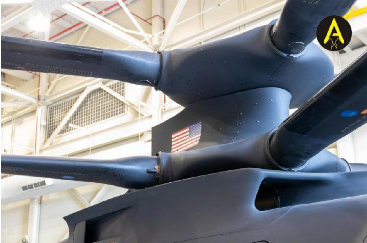
The two main rotors' heads and the fairing covering the rotor mast.
