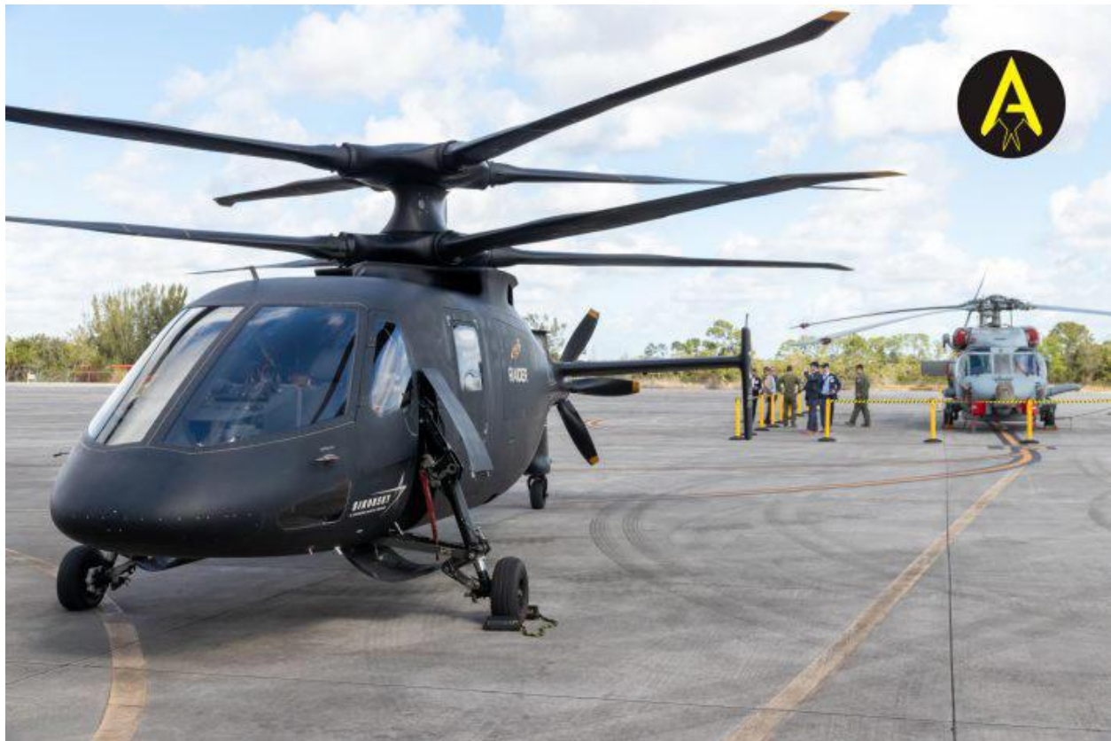
The S-97 Raider and, in the background, an MH-60R Seahawk, providing a quick comparison between the two main rotor technologies.
