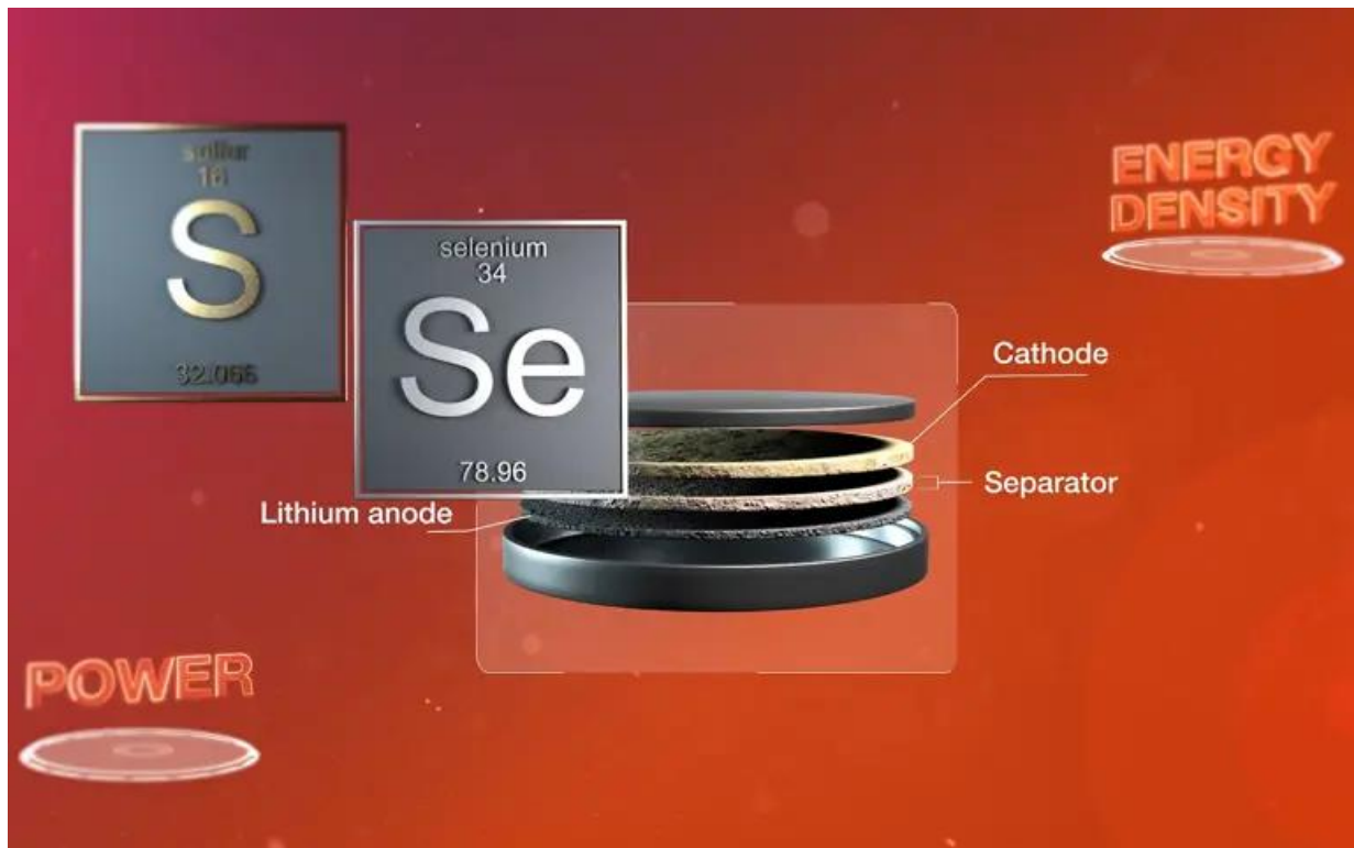
This illustration depicts the inside of a cell used in SABERS's solid-state battery, which is made primarily from sulfur and selenium. Unlike lithium-ion batteries, these cells can be stacked on top of one another without encasings to separate them. (CREDIT: NASA)© The Brighter Side of News
