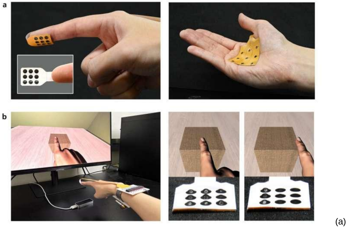
Thin flexible haptic patch for fingertip and palm of the hand. (b) VR scenario with synchronized contact geometry of virtual box. Credit: Hee-kyung Kwon
