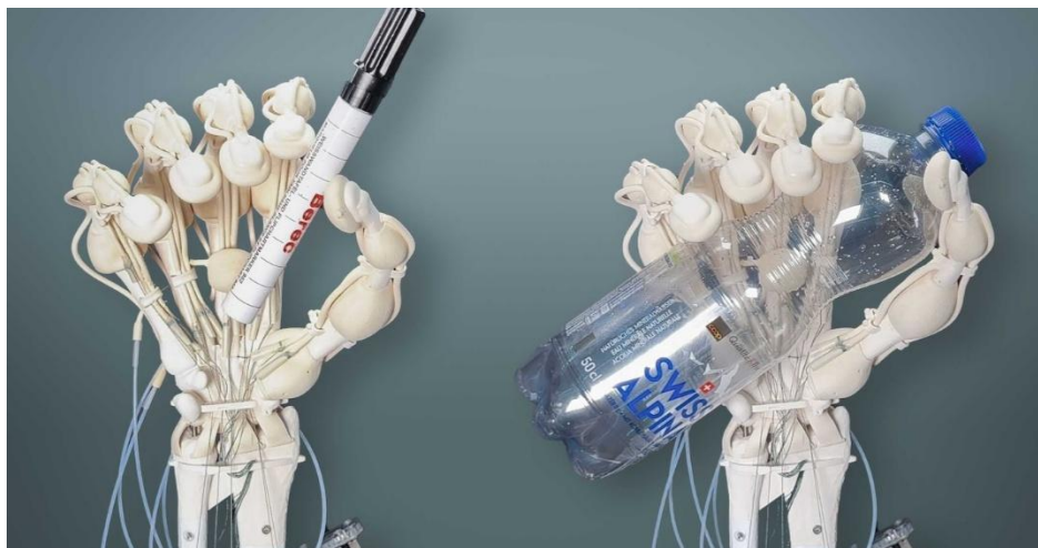
An image montage of the soft robotic hand holding a marker pen and a water bottle. (Image credit: ETH Zurich/Thomas Buchner)
