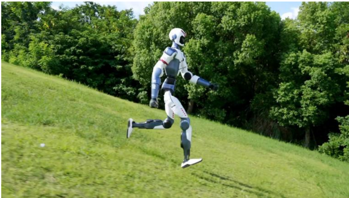
The robot has 26 joints to allow for flexible movement. Unitree Robotics
