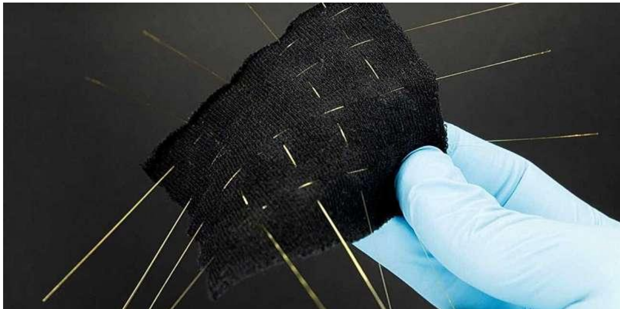
Example of a smart textile woven with glass fibers. Credit: Yingqiang Wang / ETH Zurich
