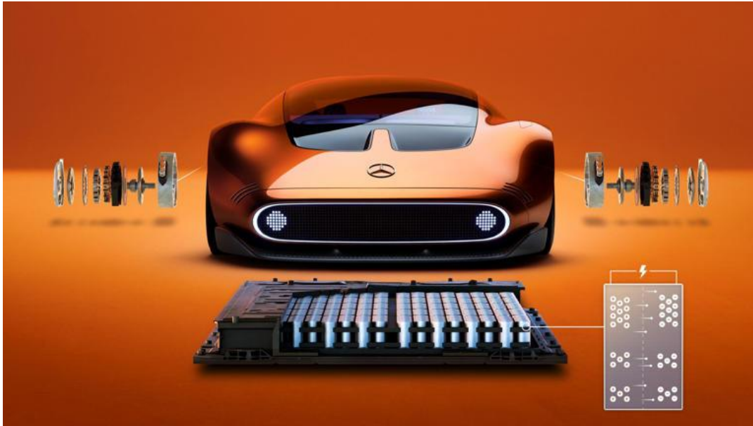
A front rendering of the Mercedes-Benz Vision One Eleven Concept, its motors and battery pack© Provided by TopSpeed
