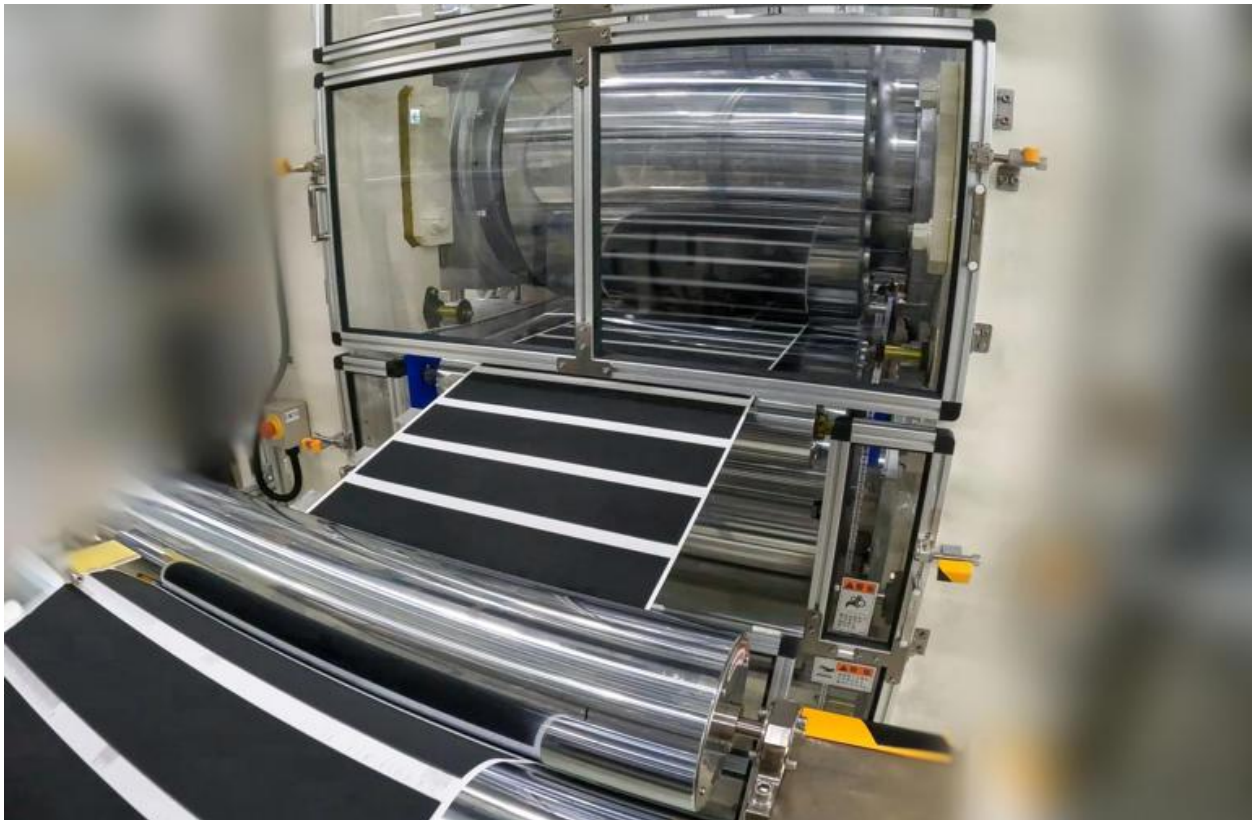
Roll pressing of cathode for solid-state batteries. © Image: Honda
