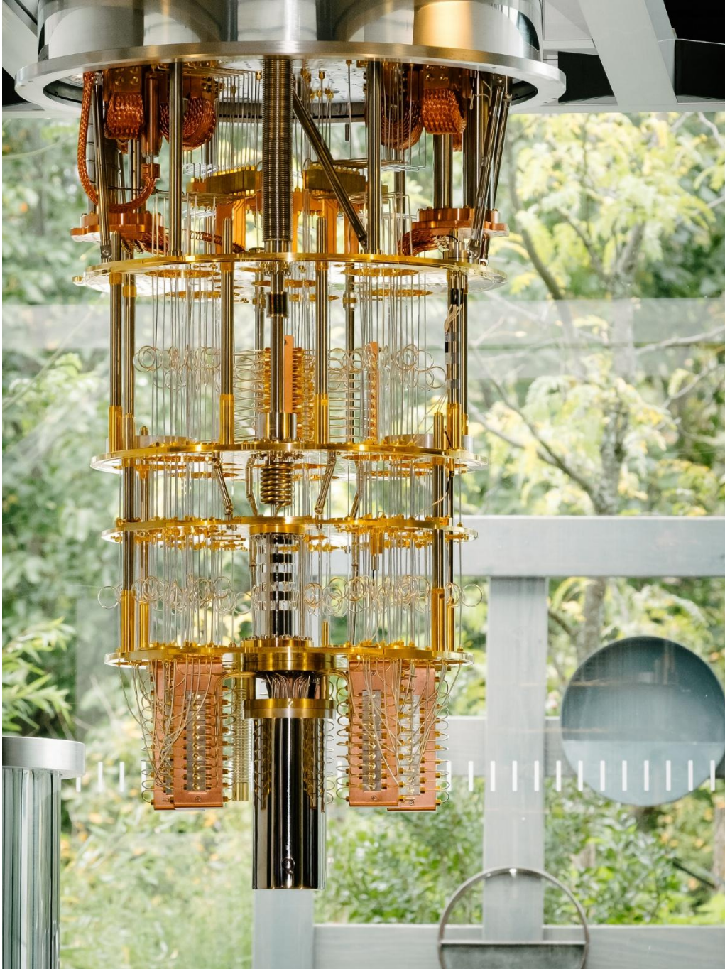
Inside one of IBM's cryostats wired for a 50-qubit quantum system. Connie Zhou for IBM
