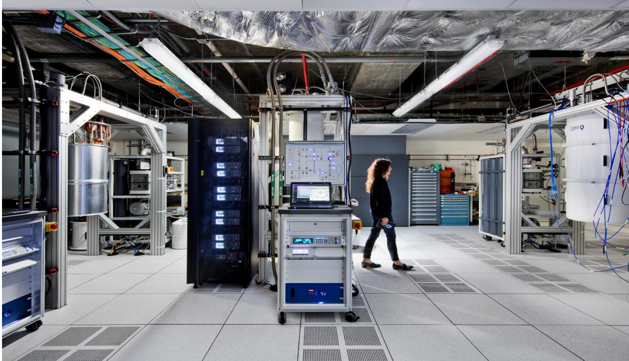
IBM's quantum computing center at the Thomas J. Watson Research Center in Yorktown Heights, New York, holds quantum computers in large cryogenic tanks (far right) that are cooled to a fraction of a degree above absolute zero.
