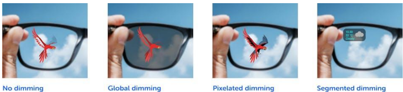
FIGURE 2. Pixelated dimming is essential for clear virtual objects in bright light.
