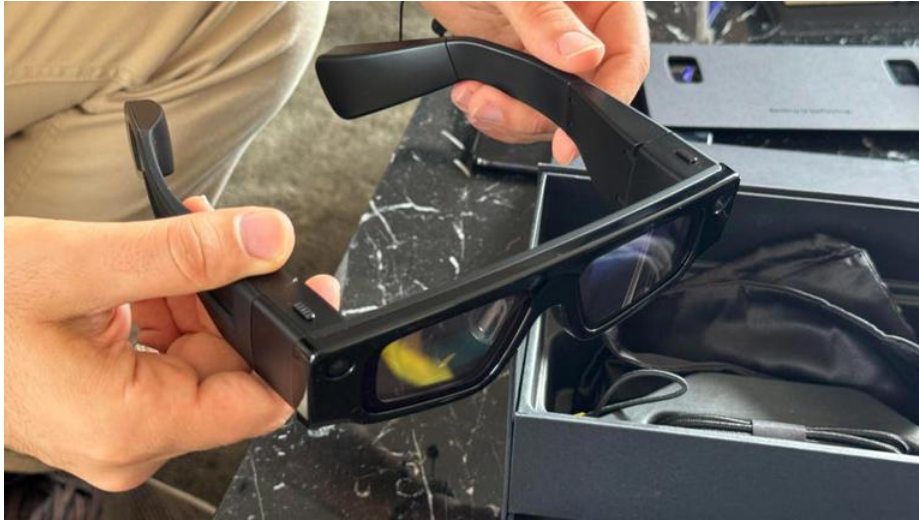
The new Spectacles have thick arms that contain the processors, projectors and batteries. Scott Stein/CNET
