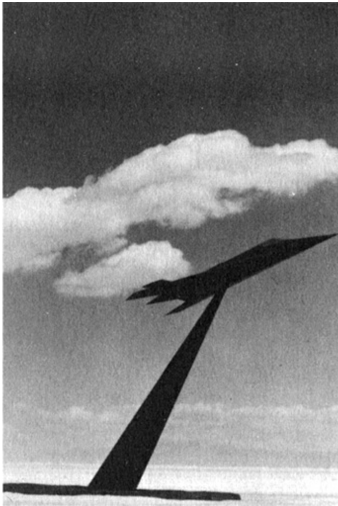
Model of the Stealth fighter undergoing radar testing at White Sands, New Mexico. The test results were so spectacular that the Air Force tamped on the tightest security lid since the atomic bomb. ( U.S. Air Force )
