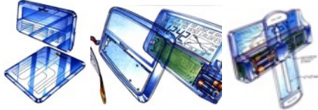
Relaxor – 1987, Santa Fe Springs, CA, invention, design-engineering and prototyping of a graphing scale that keeps track of your weight over time.
