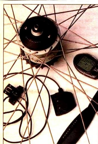
Power-Tap is a new, economical device for measuring power and other physiological data that can be mounted on most road or mountain bikes.
