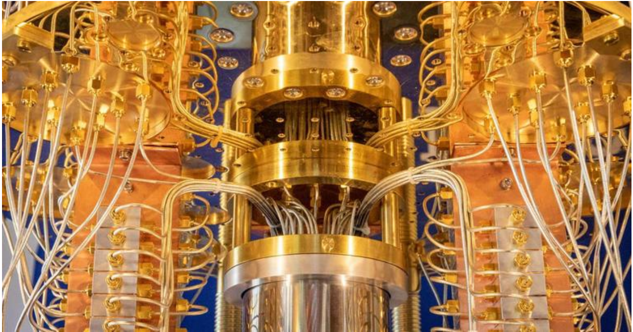
A close-up view of an IBM quantum computer. The processor is in the silver-colored cylinder. Stephen Shankland/CNET
