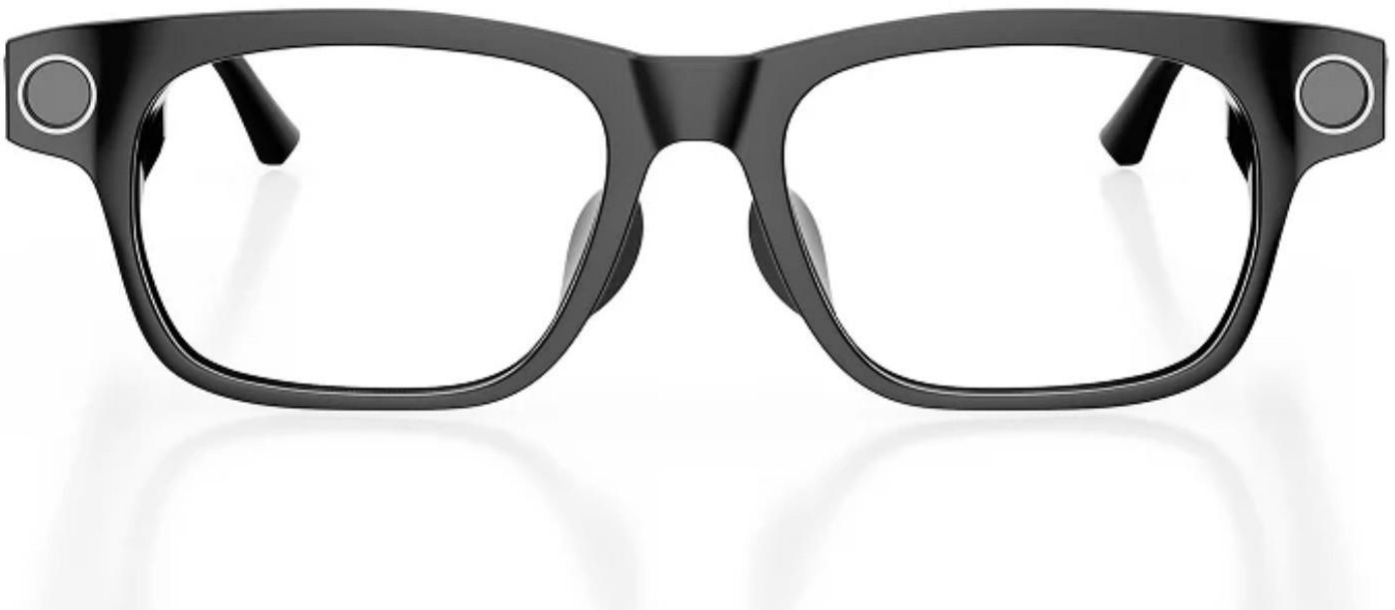
This view of the Ally Solos glasses shows the cameras located on each side of the frame. Image: Envision
