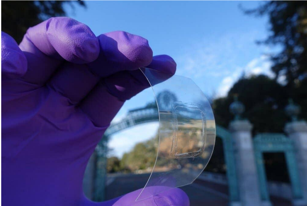
Applying mechanical strain on this atomically thin, transparent monolayer semiconductor results in a material with near 100% light-emission efficiency. (Credit: Ali Javey/Berkeley Lab)
