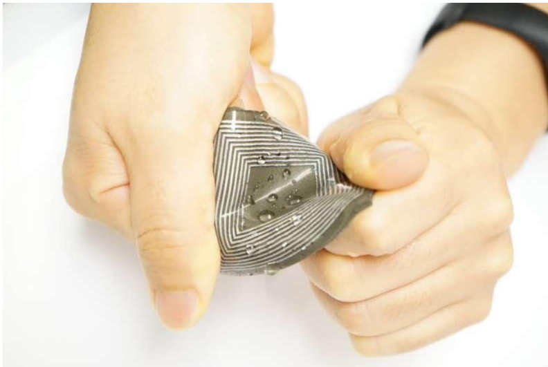
UCLA-designed self-powered, stretchable, waterproof magnetoelastic generator for bioelectronics. (Credit: Jun Chen/UCLA)
