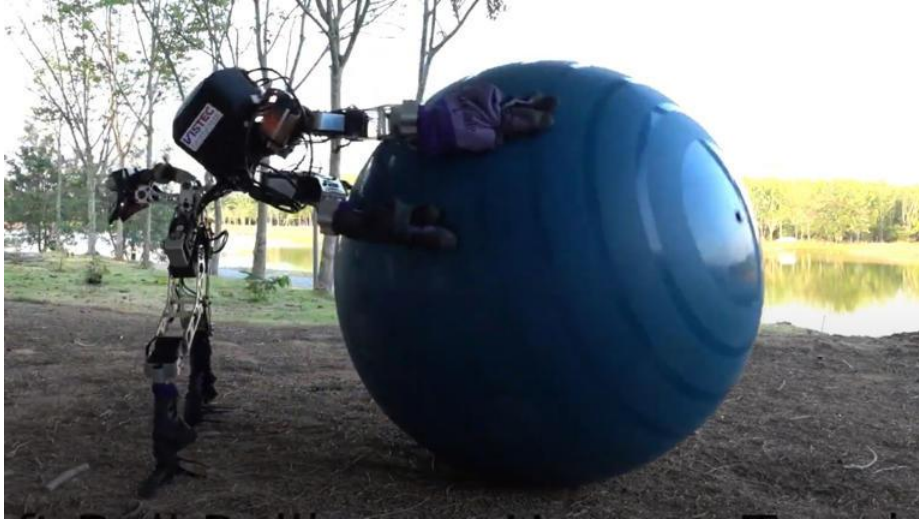
Dung beetle-inspired robot masters object rolling with adaptive leg control
