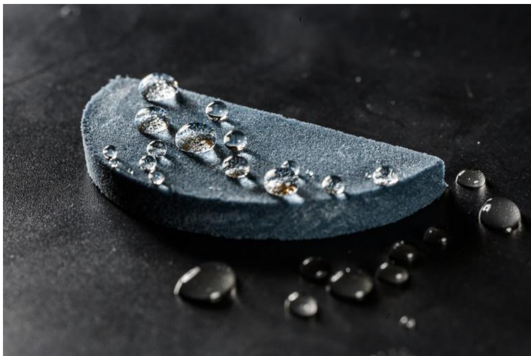
Aerogel can obtain high hydrophobicity by simple chemical modifications. Credit: Thor Balkhed© Provided by Phys.org
